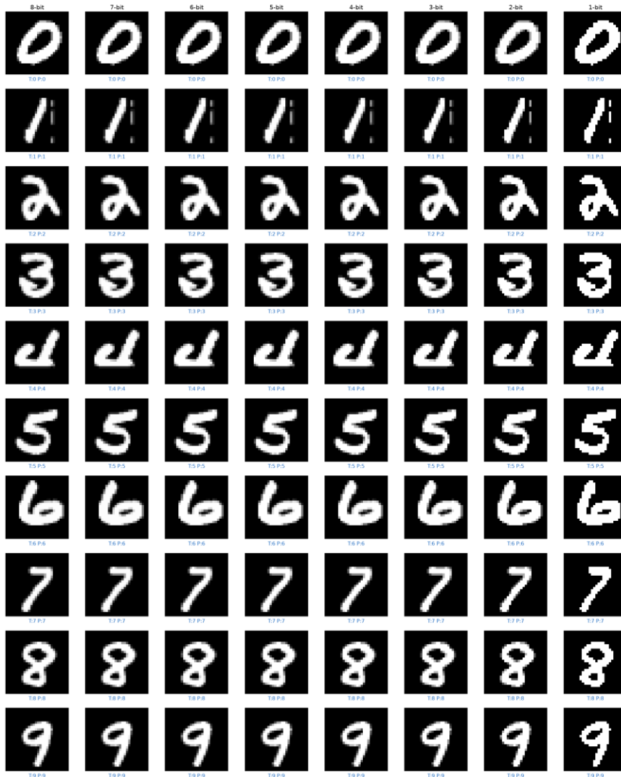
Input Quantization Effect on Images (Weights: int8, no quantization)
